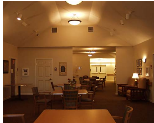
Figure III The dining and activity areas of this Alzheimer's Care Facility had very low light levels (between 70 – 180 lux) with very little daylight.
