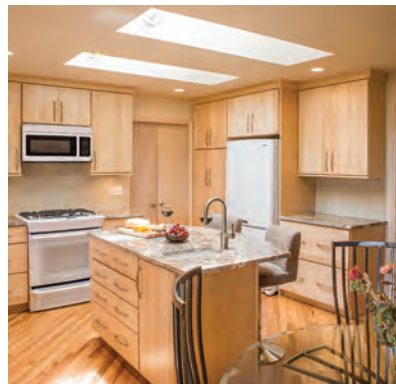
LEFT: Limited daylight and poor electric lighting. Dark colors on the soffit above the cabinets and dark floors absorb the light. RIGHT: Kitchen was remodeled to include skylights that provide abundant daylight. Recessed downlights and surface-mounted directional lighting provides light to the island and countertops. Light-colored flooring and cabinetry reflect light in the space. (Photos courtesy of Doug Walter Architects)
