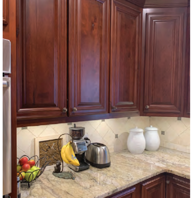
LEFT: No under-cabinet lighting. RIGHT: Under-cabinet lighting mounted on the front edge of upper-wall cabinets, providing the needed task lighting. Fixtures are available with cord and plug or hard wired, and in variable CCTs and with dimmers. (Photos courtesy of Rebecca Hadley- Catter)
