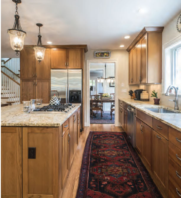
Recessed downlights can be used to provide task lighting on the countertop and inside the cabinets, and to illuminate the circulation areas. (Photo courtesy of Doug Walter Architects)
